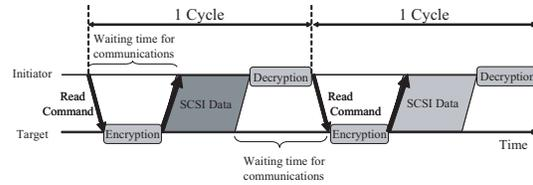
Figure 1. iSCSI Sequential Read Access with an Encryption in the Upper-layer
