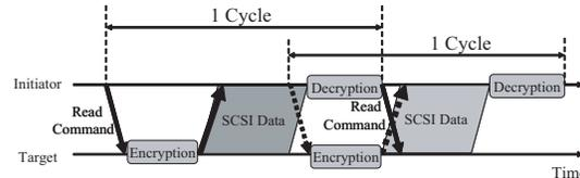
Figure 2. iSCSI Sequential Read Access with an Optimization of Encryption Processing in the Upper-layer
