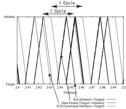
Figure 11. TCP packet transfer : our system (two processes)
