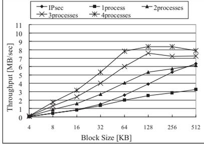
Figure 6. Throughput in 8ms Latency Network
