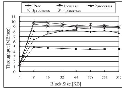
Figure 4. Throughput in a No-latency Network
