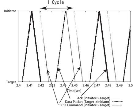
Figure 10. TCP packet transfer : our system (a single process)
