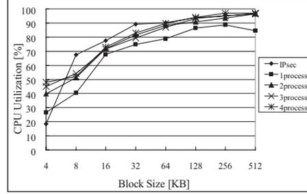
Figure 7. CPU Utilization in a No-latency Network (Target)
