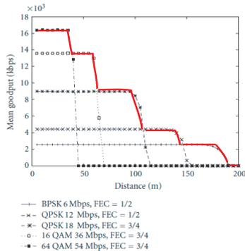
Figure 1: Throughput in multi-rate by simulation
