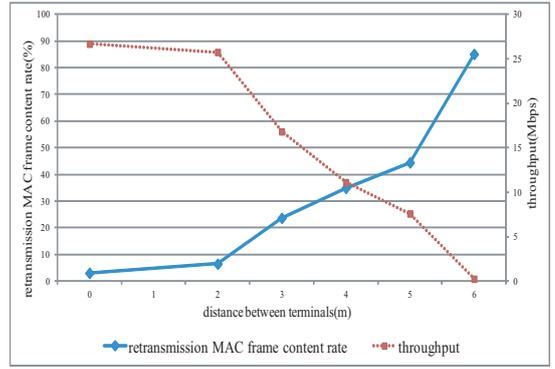
Figure 6: Retransmission MAC frame content rate vs. throughput
