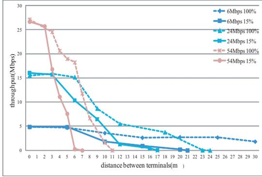
Figure 5: Throughput with radio emission powers of 15 % and 100 %
