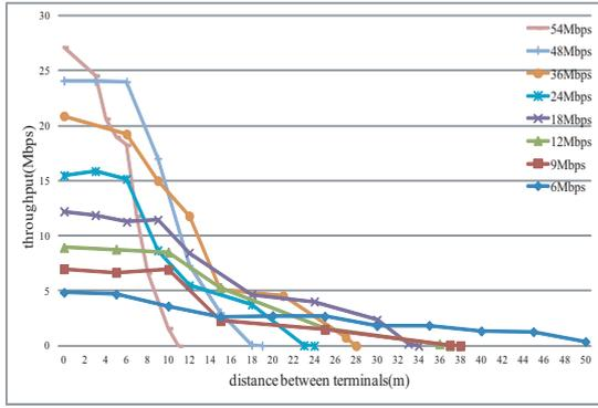
Figure 4: Throughput for distance in multi-rates
