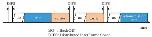
Figure 2: Example behavior of CSMA/CA with carrier from other wireless LAN
