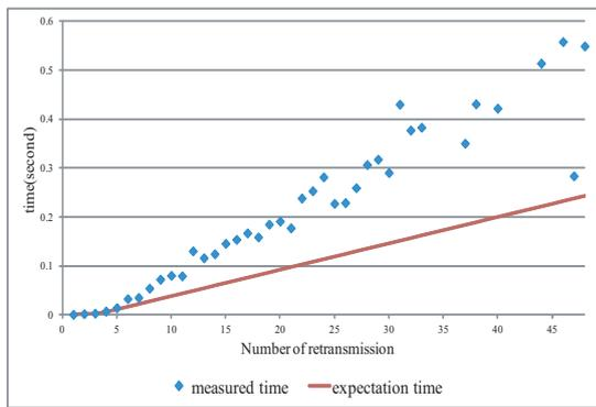
**Figure 8: Measured inter-arrival and expectation retransmission times**
